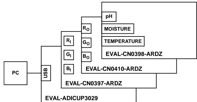
Figure 4. Smart Greenhouse System Functional Block Diagram
