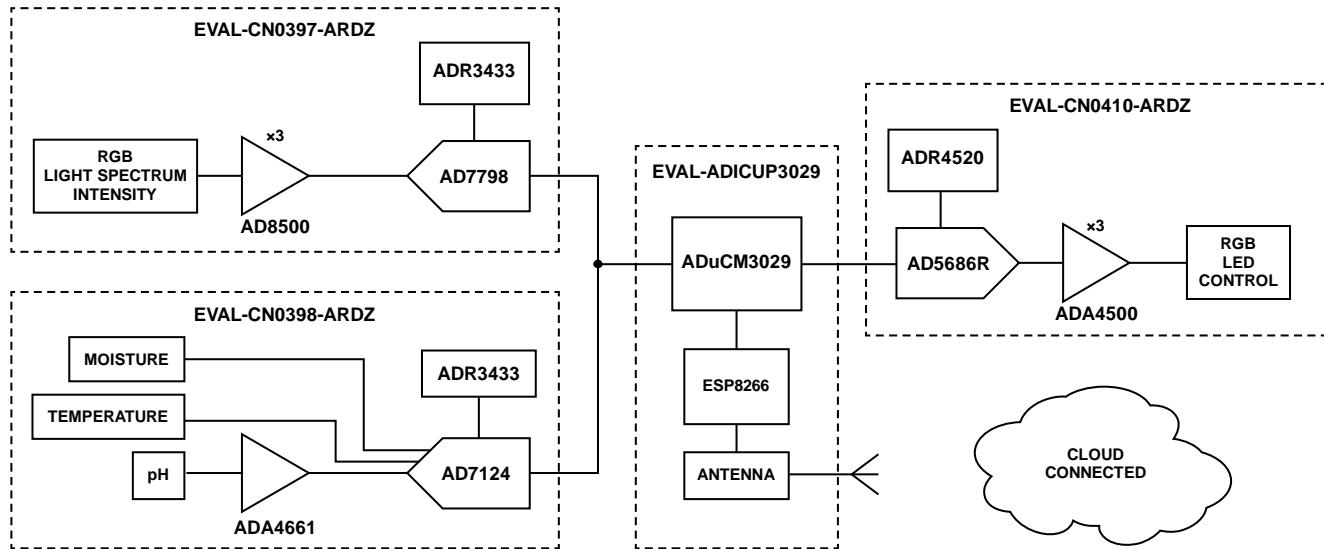
Figure 1. Simplified System Block Diagram
