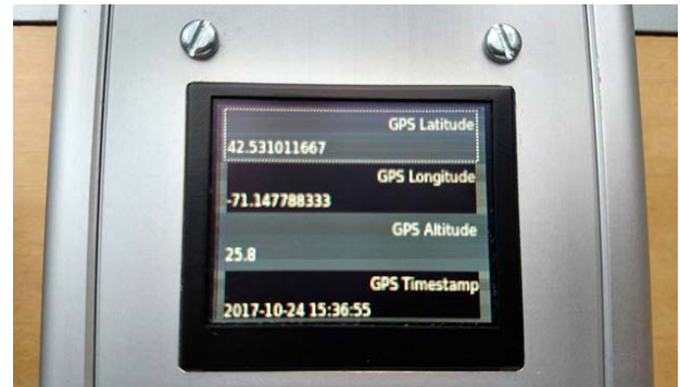
Figure 14. OLED Showing GPS Coordinates on an ADRV-PACKRF
