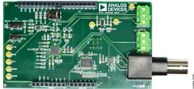
Figure 9. [EVAL-CN0398-ARDZ](#) Shield Board
