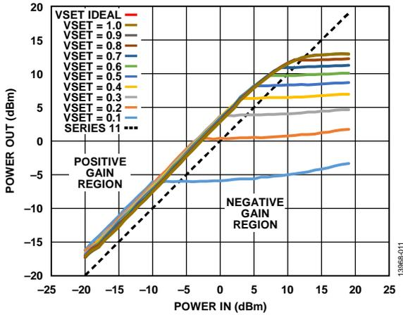
Figure 11. ADL6010 AGC Loop Measured Performance at 37.5 GHz
