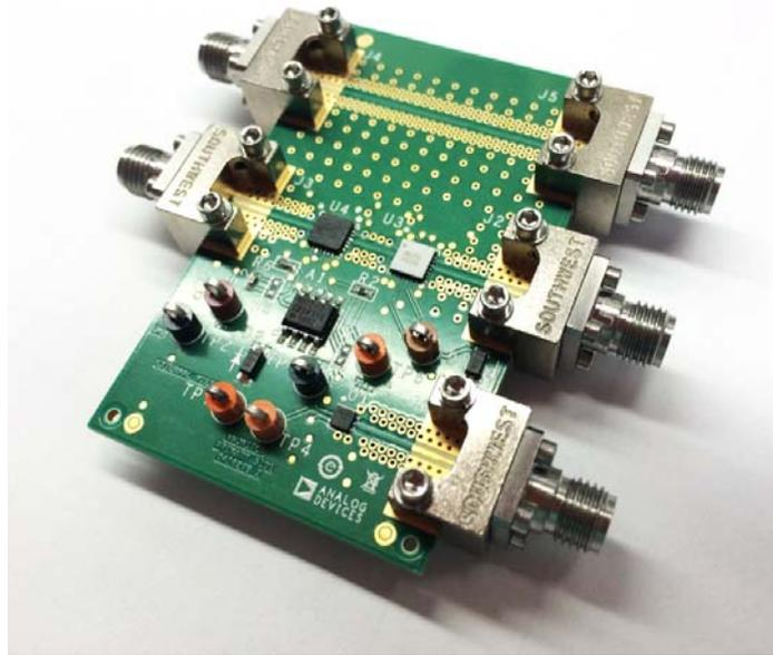
Figure 2. EVAL-CN0390-EB1Z AGC Printed Circuit Board (PCB) Photo
