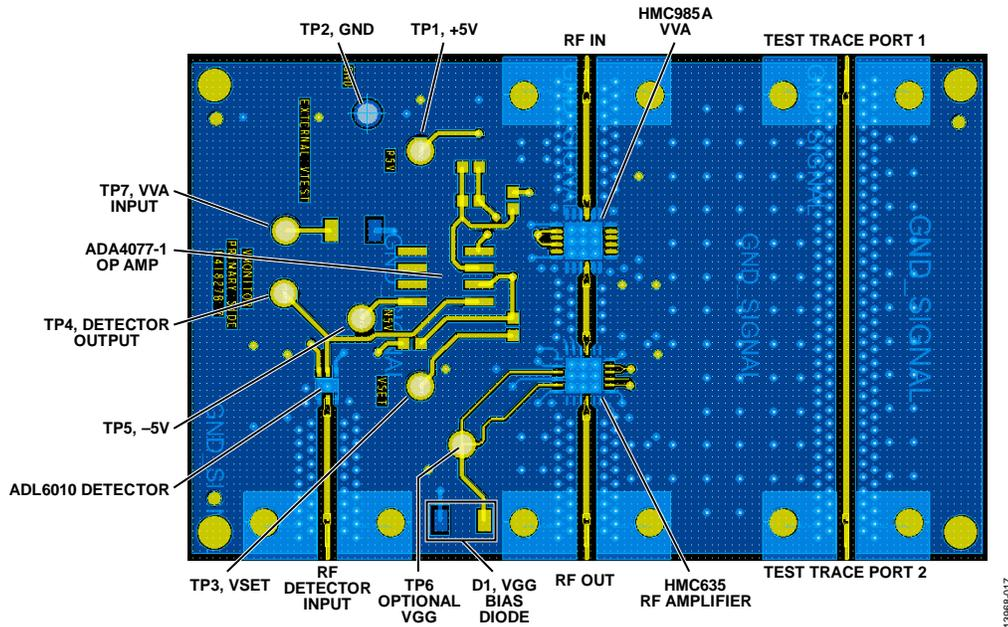
Figure 17. ADL6010 AGC Circuit—PCB
