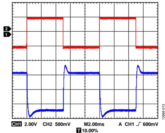
Figure 13. Transient Response with Step Applied to VSET
