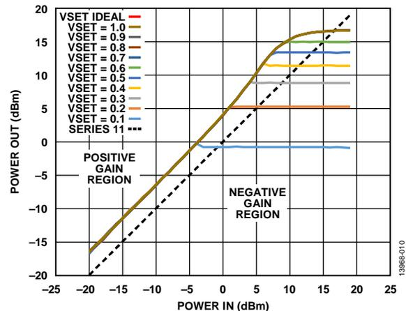
Figure 10. ADL6010 AGC Loop Measured Performance at 30 GHz
