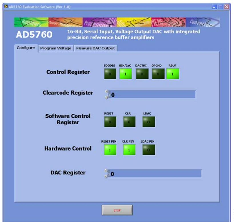
Figure 6. Evaluation Software Main Window
