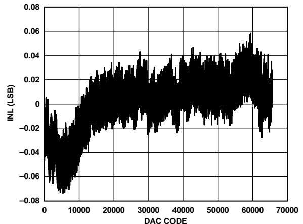
Figure 2. Integral Nonlinearity vs. DAC Code
