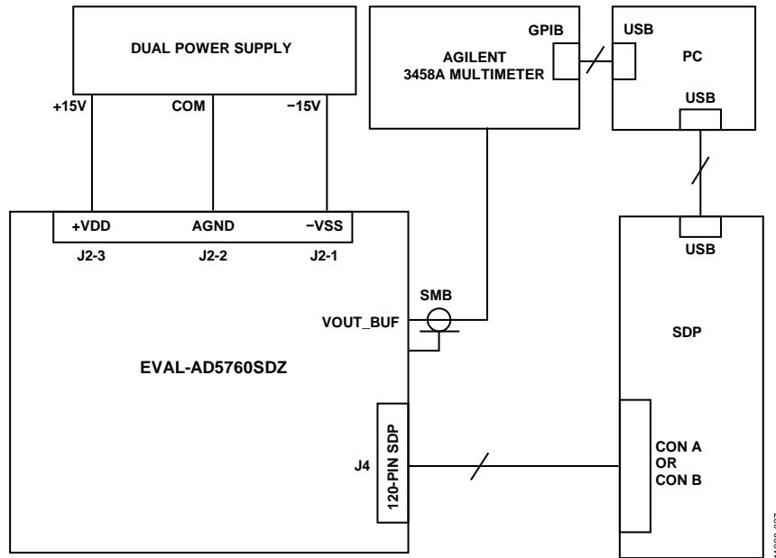
Figure 7. Functional Block Diagram of Test Setup
