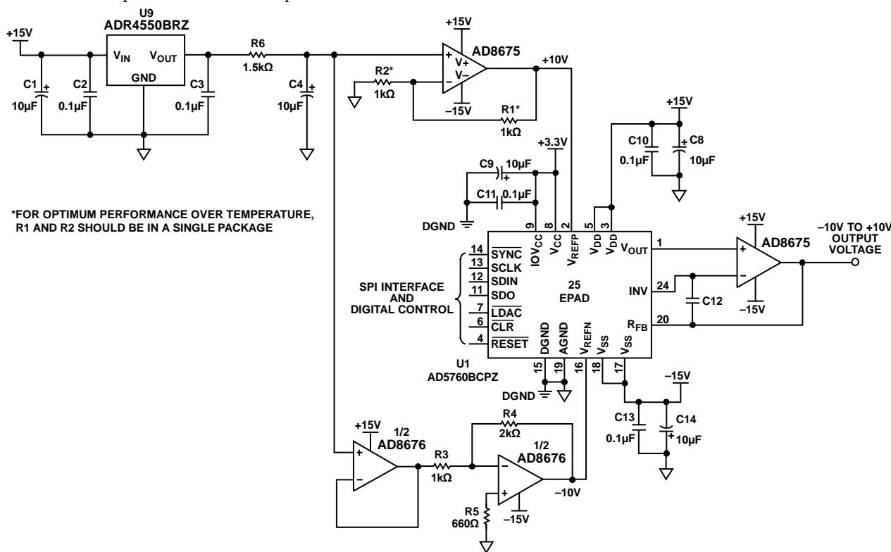
Figure 1. 16-Bit Accurate,  $\pm 10$  V Voltage Source (Simplified Schematic: All Connections and Decoupling Not Shown)
