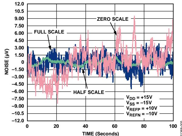
Figure 5. DAC Output Voltage Noise Measured Over 100 Second Period for Full Scale (Blue), Half Scale (Green), and Zero Scale (Red) with [ADR4550](#) Voltage Reference for a 20 V Peak-to-Peak Bipolar Output Voltage Range
