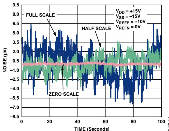
Figure 4. DAC Output Voltage Noise Measured Over 100 Second Period for Full Scale (Blue), Half Scale (Green), and Zero Scale (Red) with [ADR4550](#) Voltage Reference for a 10 V Peak-to-Peak Unipolar Output Voltage Range
