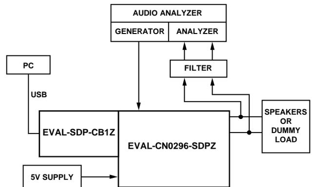
Figure 4. Sound Bar Test Setup Device Configuration
