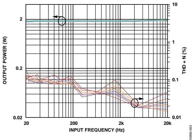
Figure 3. Output Power and THD+N vs. Input Frequency
