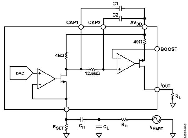
Figure 3. AD5420/AD5410 and AD5700 HART Modem Connection
