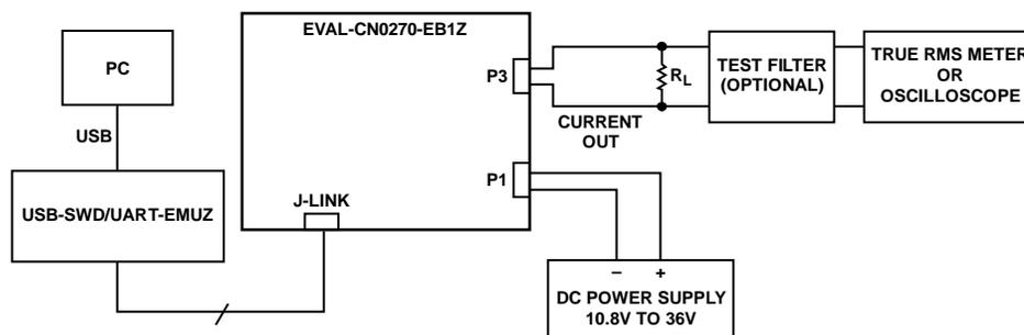
Figure 11. Test Setup Block Diagram
