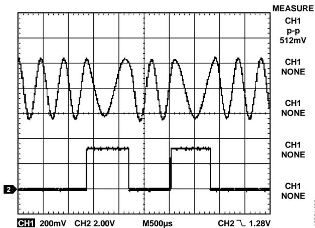
Figure 5. FSK Waveforms Measured Across a 500  $\Omega$  Load
