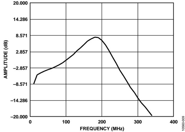
Figure 9. Antialiasing Filter Response,  $f_c = 183$  MHz
