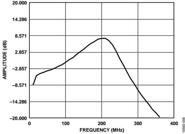
Figure 6. Antialiasing Filter Response,  $f_c = 203$  MHz
