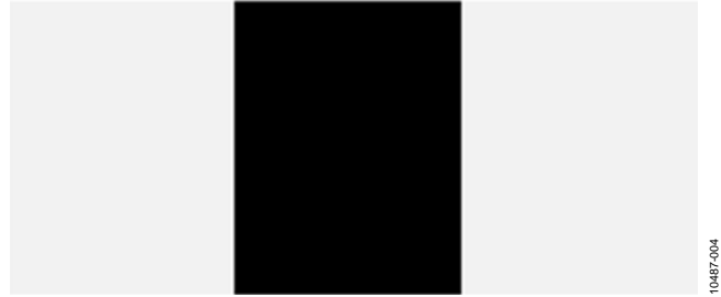
Figure 4. Video Display of Black Stripe Showing 1 V p-p, 500 kHz Common-Mode Noise Rejected by the ADA4830-1
