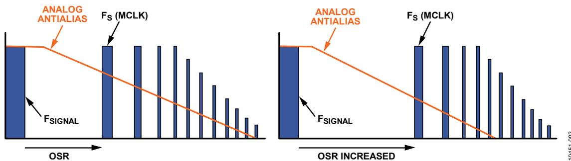
Figure 2. Increasing Oversampling Ratio (OSR) Reduces Noise
