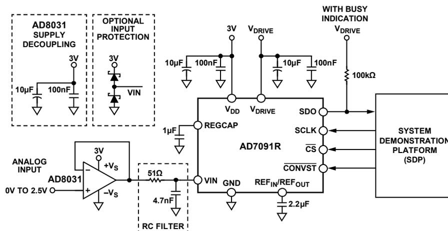
Figure 1. 12-Bit, 1 MSPS Low Power ADC with Driver (Simplified Schematic: All Connections Not Shown)
