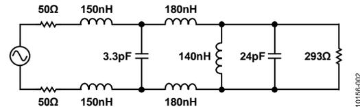
Figure 2. Final Design Values for Fifth-Order Differential Butterworth Filter with  $Z_s = 100 \Omega$ ,  $Z_L = 293 \Omega$ ,  $f_c = 182.5 \text{ MHz}$
