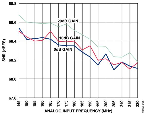
Figure 5. SNR Performance vs. Analog Input Frequency (0 dB Gain, 10 dB Gain, and 20 dB Gain)
