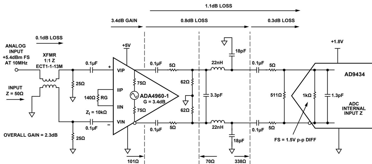
Figure 1. 12-Bit, 500 MSPS Wideband Receiver Front End (Simplified Schematic: All Connections and Decoupling Not Shown)
