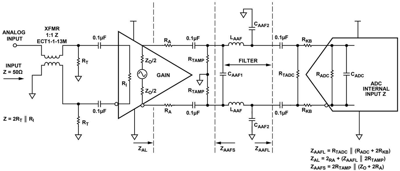
Figure 5. Generalized Differential Amplifier/ADC Interface with Low-Pass Filter
