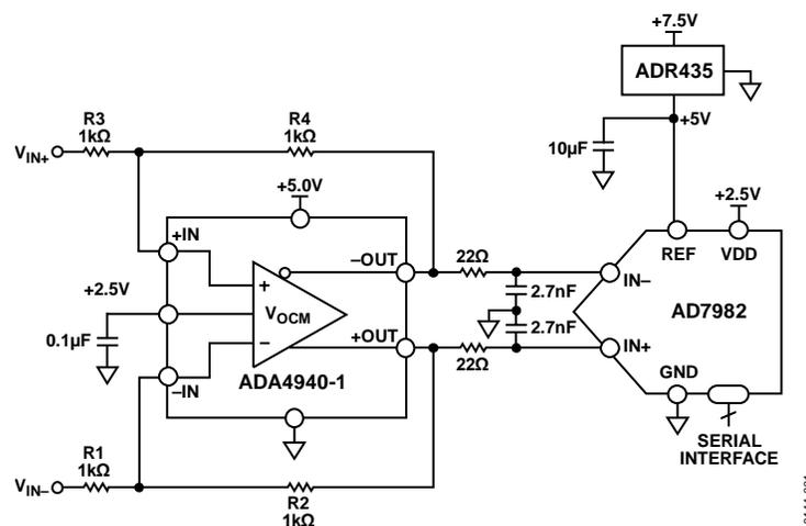
Figure 1. High Performance 18-Bit Differential ADC Driver (Simplified Schematic: All Connections and Decoupling Not Shown)
