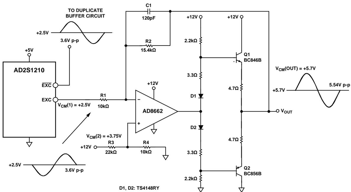
Figure 1. High Current Buffer for the AD2S1210 RDC Reference Signal Output (Simplified Schematic: All Connections and Decoupling Not Shown)
