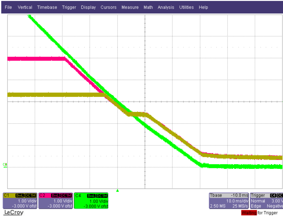
Figure 9. Switching regulator turn off at no load: Ch1 = 3.3 V, Ch2 = 5.0 V, Ch4 = Vin
