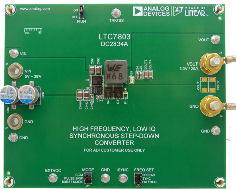
Figure 3. DC2834A demo board.
