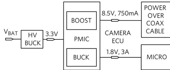
Figure 4. Power PMIC Inside the Camera ECU
