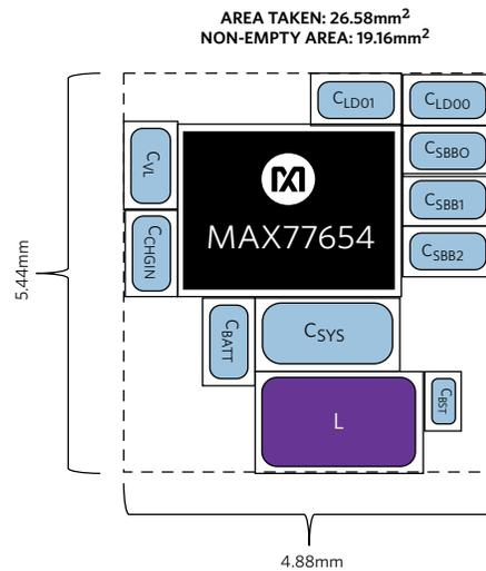
Figure 6. SIMO PMIC Solution with Minimal Board Space (19.2mm<sup>2</sup>)
