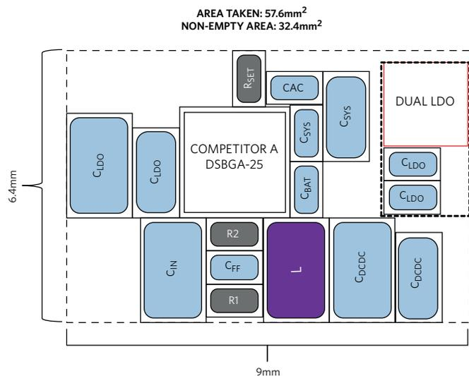
Figure 10. Board Space of a Typical Wearable Solution (32.4mm<sup>2</sup>)
