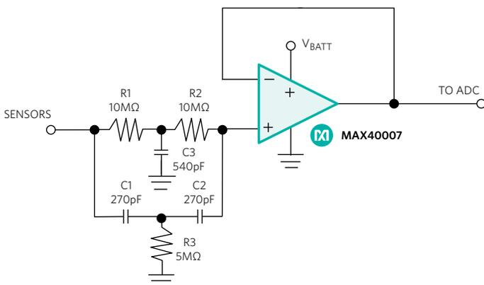
Figure 3. A 60Hz Notch Filter Uses One Amplifier and Several Resistors and Capacitors
