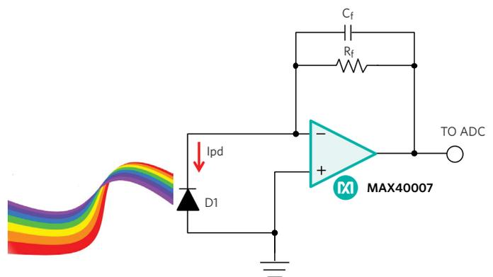
Figure 5. Nanopower Photodetector Circuit Uses Three Components and One Amplifier
