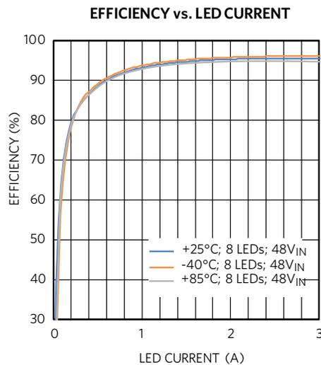
Figure 6. LED Driver Solution Efficiency vs. Load Current
