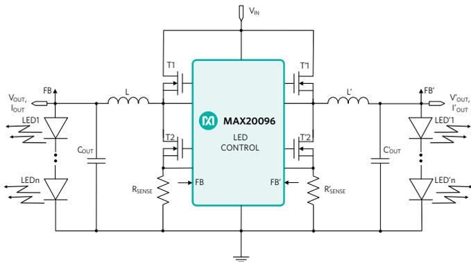
Figure 4. Synchronous High-Power Dual-Buck LED Controller
