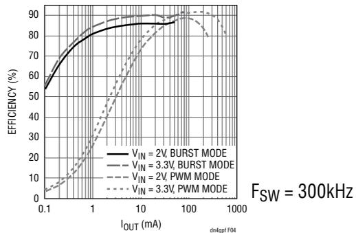
**Figure 4. With a Lower Switching Frequency and a Larger Inductor, a Smaller Battery Can Be Used. Efficiency Gain Up to 30% in the 1mA to 10mA Load Range (in PWM Mode) Can Significantly Improve Applications That Operate with Light Loads.**
