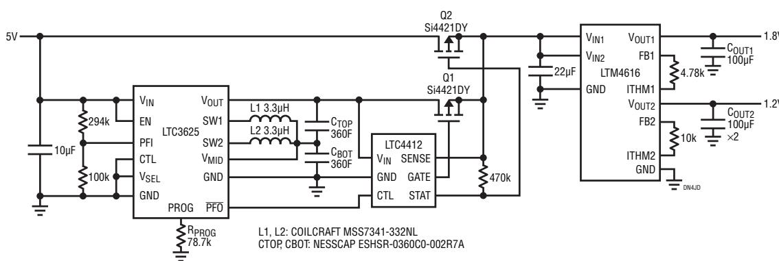
Figure 1. Supercapacitor Energy Storage System for Data Backup
