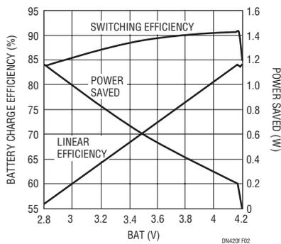
**Figure 2. Switching PowerPath Battery Charger Efficiency and Power Savings Relative to a Linear Charger. ( $V_{BUS} = 5V$ , 5X MODE,  $R_{CLPROG} = 2.94k$ ,  $R_{PROG} = 1k$ ,  $I_{BAT} = 0.7A$  at  $V_{BAT} = 2.8V$ )**
