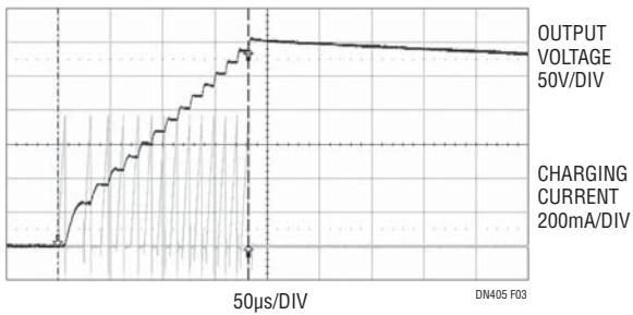
**Figure 3. LT3750 Charges 0.1 $\mu$ F to 300V in 180 $\mu$ s**
