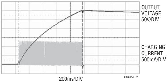
**Figure 2. LT3750 Charges 400 $\mu$ F to 300V in 0.92 Seconds**
