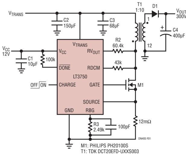
**Figure 1. LT3750 Circuit Charges 400 $\mu$ F Capacitor to 300V.
