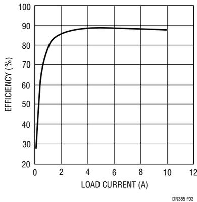
**Figure 3. Efficiency of the Application in Figure 2**
