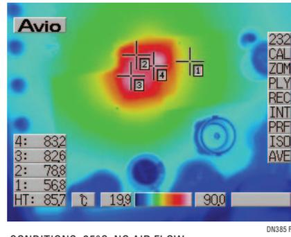
**Figure 4. The LTM4600 Exhibits Impressive Thermal Performance, Even Without Air Flow and Heat Sink (24V to 3.3V at 10A, Top View). For a Color Representation, Download the File at [www.linear.com](http://www.linear.com)**
