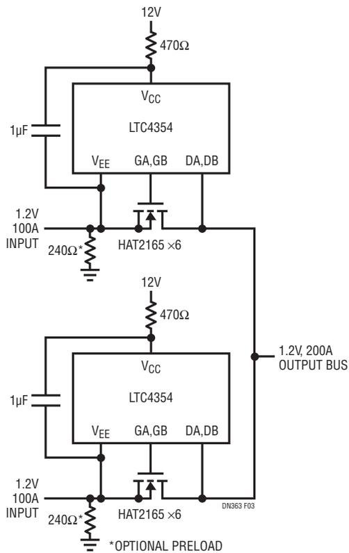
**Figure 3. Positive Low Voltage Diode-OR Combines Multiple Switching Converters**
