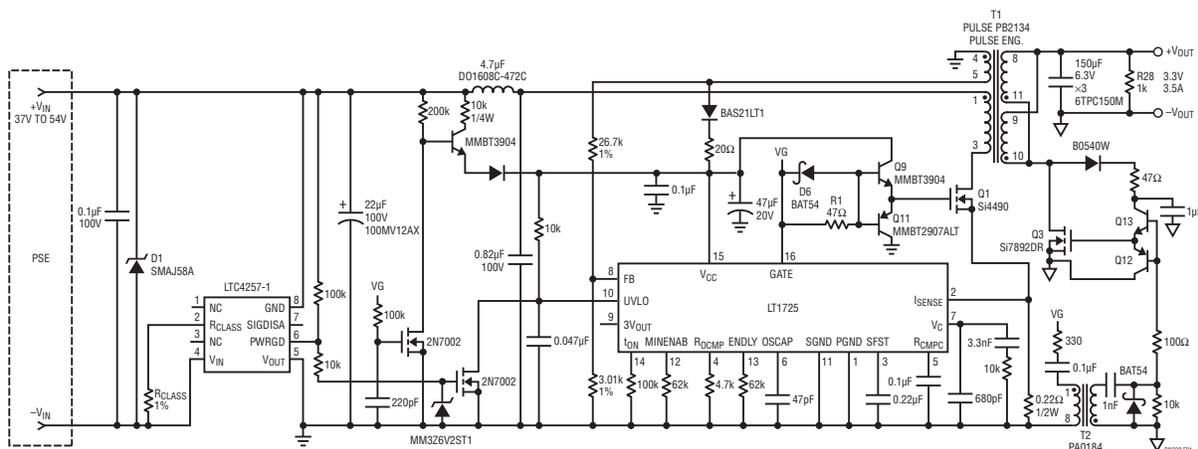
Figure 1. 36V-72V Input to 3.3V at 3.5A Output, Isolated Synchronous Flyback Converter
