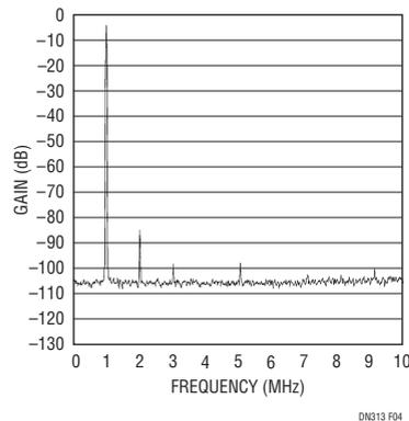
**Figure 4. Spectral Plot of a 1MHz, 2V<sub>P-P</sub>, Differential Sine Wave Input to an LT6600-10 Filter Plus an LT1744 14-Bit ADC (a DC to 10MHz Plot of a 4096-Point Averaged FFT with a 50MHz Sample Rate)**
