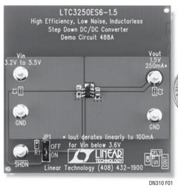
**Figure 1.** The LTC3250 Is Available in a Tiny 6-Pin ThinSOT Package Making it Possible to Fit a Complete Converter in Less Than 0.04in<sup>2</sup>
