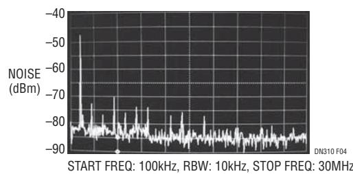
Figure 4. Conventional Step-Down Regulator Output Noise Spectrum with 22µF Output Capacitor ( $I_0 = 500\text{mA}$ )
