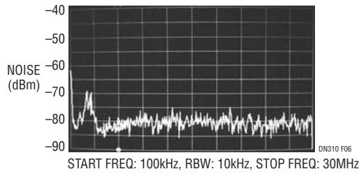
Figure 6. LTC3251 Output Noise Spectrum with 10µF Output Capacitor ( $I_0 = 500\text{mA}$ )
