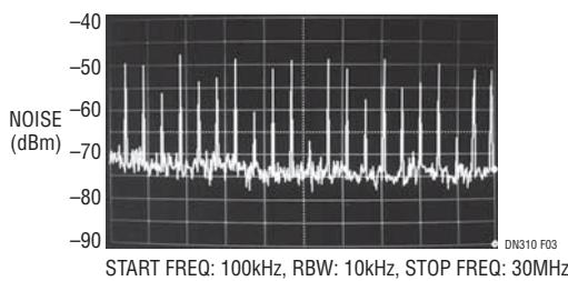
Figure 3. Conventional Step-Down Regulator Input Noise Spectrum with 10µF Input Capacitor ( $I_0 = 500\text{mA}$ )
