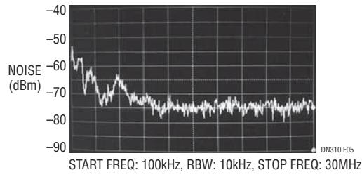
Figure 5. LTC3251 Input Noise Spectrum with 1µF Input Capacitor ( $I_0 = 500\text{mA}$ )
