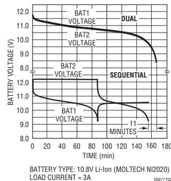
Figure 2. Dual Discharge Extends Run Time
