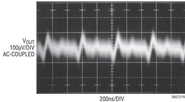
**Figure 2. 50V Avalanche Photodiode Bias Shows 200 $\mu$ V<sub>P-P</sub> Ripple and Noise, Improving Fiber Optic Receiver Sensitivity**
