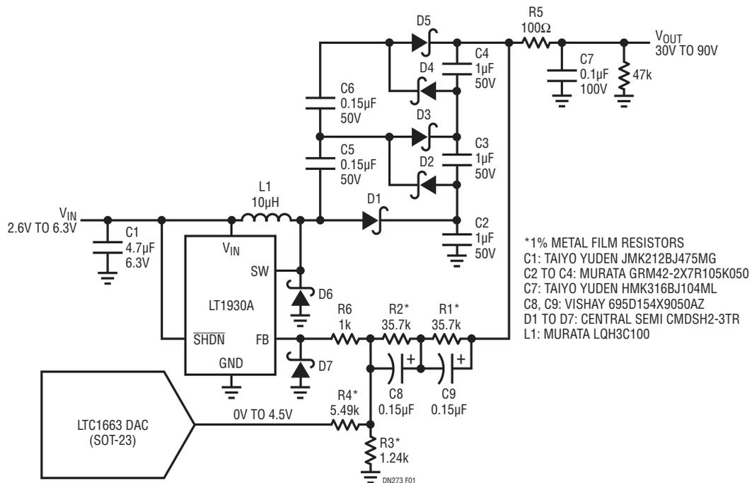
**Figure 1. LT1930A-Based Boost Regulator Produces 30V to 90V for Avalanche Photodiode Bias Supplies with Only 200µV<sub>p-p</sub> Noise**
