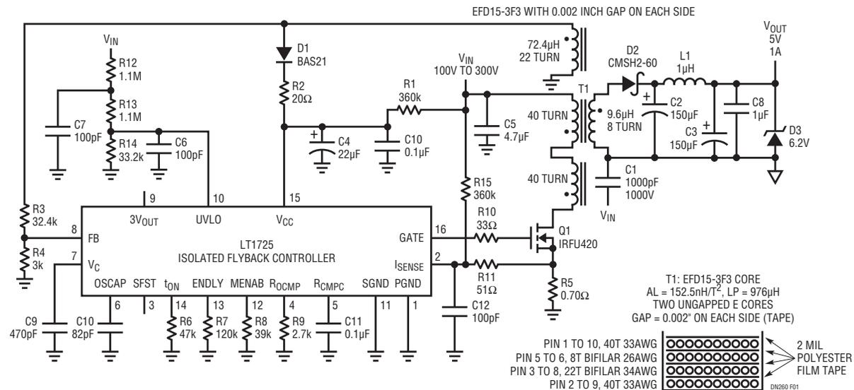
100V<sub>IN</sub> to 300V<sub>IN</sub>, 5V<sub>OUT</sub> at 1A Isolated Flyback Power Supply
