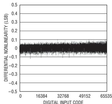
**Figure 2. The Outstanding INL and DNL ( $\leq 0.25$ LSB Typ) and Very Low Drift Allow a Maximum 1LSB Specification Over Temperature**
