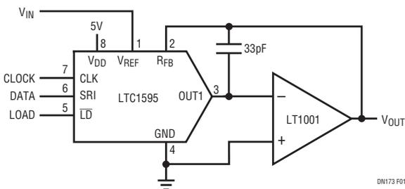
**Figure 1. With a Single Op Amp, the 16-Bit DAC Performs 2-Quadrant Multiplication with  $\pm 10$ V Input and Output Ranges. A Fixed  $-10$ V Reference Generates a Precision 16-Bit 0V to 10V Unipolar Output**
