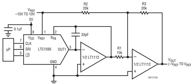
Figure 5. The LTC1595 and the LT1122 Dual Op Amp Achieve 4-Quadrant Multiplication and a 16-Bit  $\pm 10V$  Bipolar Output with 10V Reference
