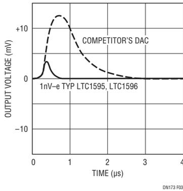
Figure 3. The Output Glitch is Less Than 1nV-s, Ten Times Less Than the Best 16-Bit Industrial DACs
