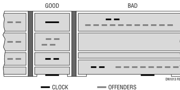
Figure 5. Example of Good and Bad Layout for Clock Routing.
