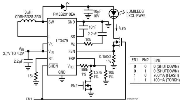
**Figure 4. The LT3479 Boost Regulator Delivers 700mA Constant-Current to the LXCL-PWF2 High Voltage Luxeon Flash with 85% Efficiency and Output Disconnect**
