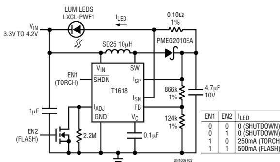
**Figure 3. The LT1618 Constant-Current, Constant-Voltage Boost Regulator can Be Configured to Give a Low Parts Count Buck-Boost Solution for LXCL-PWF1 Luxeon Flash at 500mA**
