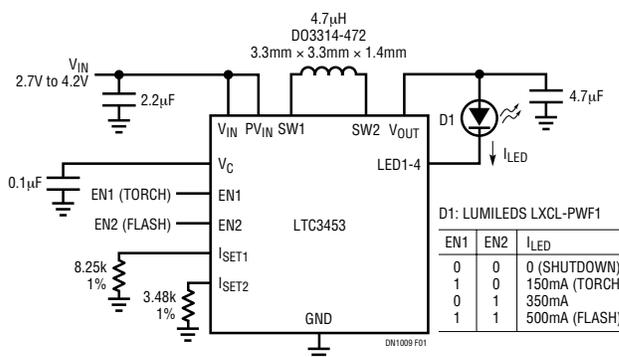
**Figure 1. High Performance LED Flash Driver Yields Greater than 90% Efficiency. The LTC3453 Buck-Boost Delivers 500mA to the LXCL-PWF1 LED Flash with Only Six Tiny External Components**
