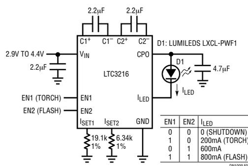
**Figure 2. This LXCL-PWF1 Luxeon Flash Driver is Extremely Small. It Requires Only an LTC3216 Low Noise High Efficiency Charge Pump in a Small DFN Package, Along with Four 0603 Capacitors and Two 0402 Resistors**
