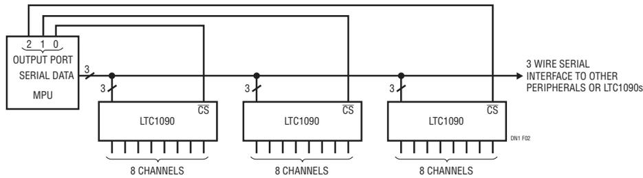
Figure 2. Several LTC1090s Sharing One 3 Wire Serial Interface
