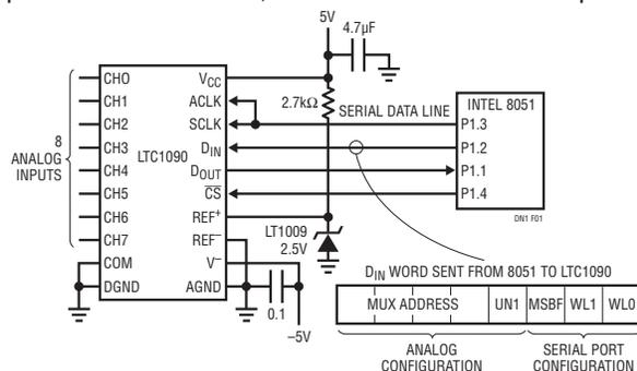
Figure 1. A Typical Hookup of the LTC1090
