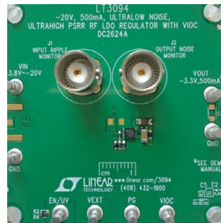
Figure 2. Demo circuit shows a tiny -3.3\ \text{V} solution.
