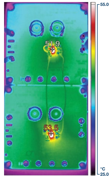
Figure 4. Thermal image of two paralleled LT3094s.
