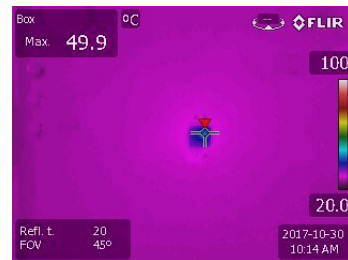
Figure 2. At Room Temperature (23°C), the LTM8074 Has Low Temperature Rise Under Full Load (12V Input to 5V Output at 1A)
