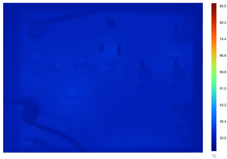
Figure 16. DC2814A-B Thermal Performance at 30V IN (Pass-Through), 30V OUT , 2.5A Load Current
