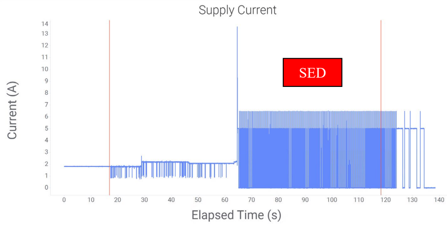
Run 27, SEL, V_{IN} = 5.3V , LET = 27.1 \text{ MeV} \cdot \text{cm}^2/\text{mg} , Hardware Mitigation
