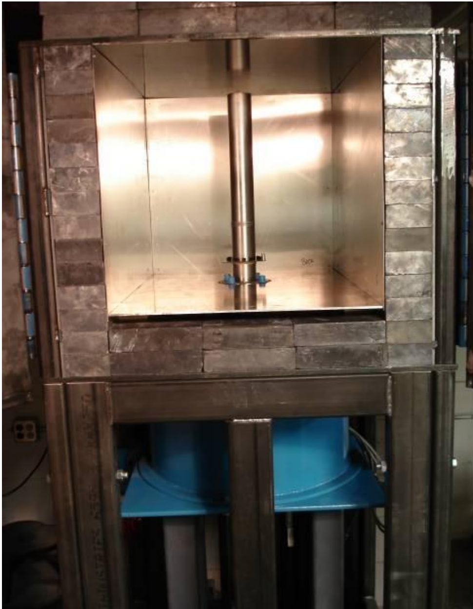
Figure 2.1. Radiation Test Solutions' high dose rate Co-60 irradiator. The dose rate is obtained by positioning the device-under-test at a fixed distance from the gamma cell. The dose rate for this irradiator varies from approximately 300rad(Si)/s close to the rods down to 1rad(Si)/s at a distance of approximately 2-feet.
