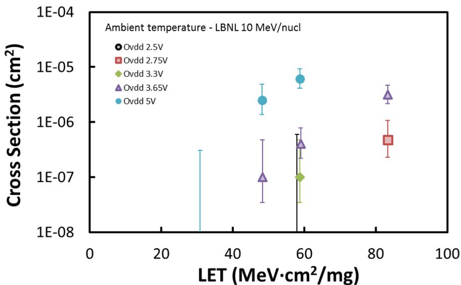
Figure 4. SEL cross section vs. LET for the RT2378 irradiated with 10 MeV/amu heavy ions.
