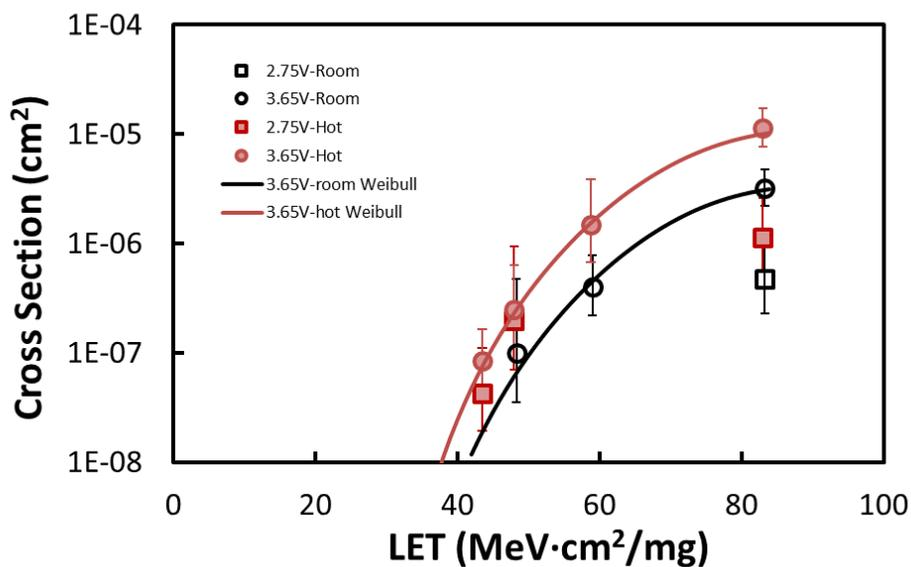
Figure 5. SEL cross section vs. LET for the RT2378 irradiated with 10 MeV/amu heavy ions.
