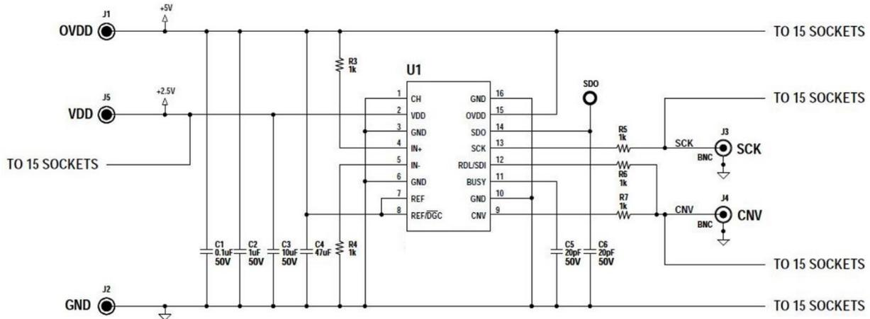
Figure 1. Circuit diagram of the SEE test circuit.
