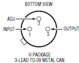
Figure B.2. H Package drawing (for reference only). This figure was extracted from Linear Technology RH117 Datasheet I.D No. 66-11-0135 Revision C.
