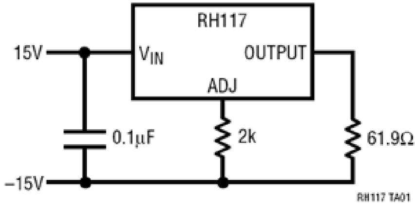
Figure B.1. Irradiation bias circuit. This figure was extracted from Linear Technology RH117 Datasheet I.D No. 66-11-0135 Revision C.
