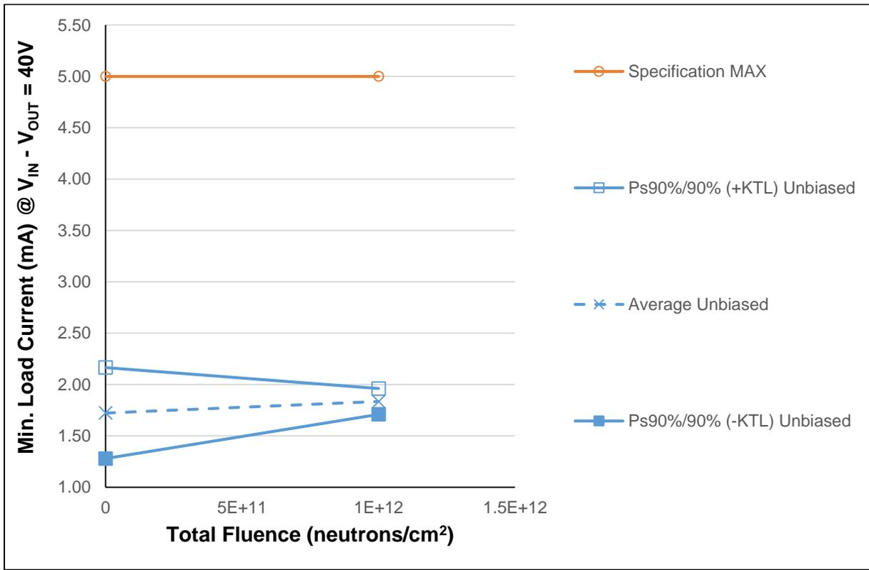
Figure 5.8: Plot of Minimum Load Current @  $V_{IN} - V_{OUT} = 40V$  versus Total Fluence
