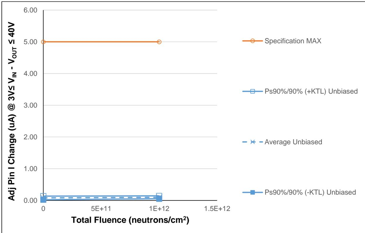
Figure 5.7: Plot of Adjust Pin Current Change @  $3V \leq V_{IN} - V_{OUT} \leq 40V$  versus Total Fluence
