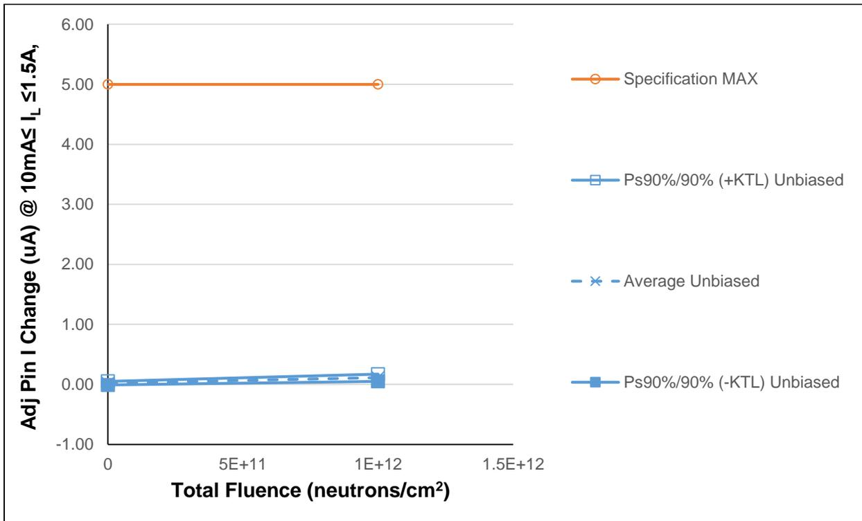
Figure 5.6: Plot of Adjust Pin Current Change @ 10mA ≤ I<sub>L</sub> ≤ 1.5A versus Total Fluence
