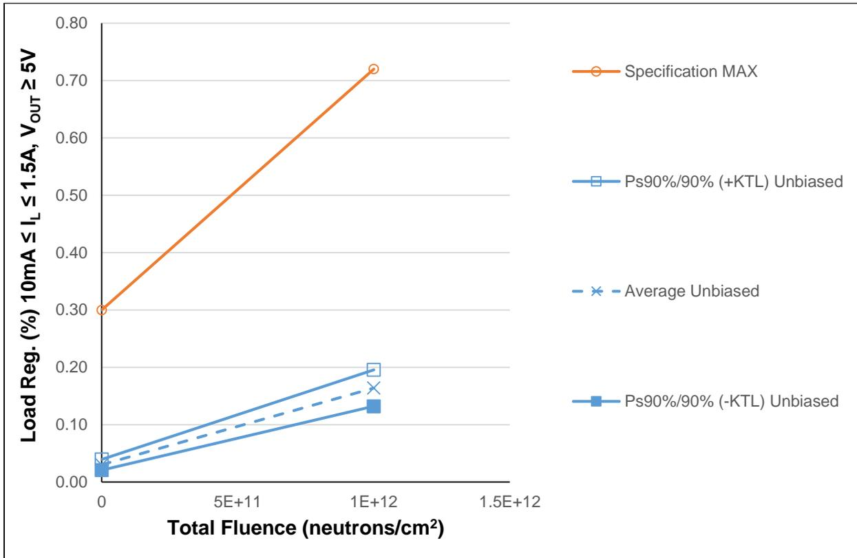
Figure 5.4: Plot of Load Regulation @  $10\text{mA} \leq I_L \leq 1.5\text{A}$ ,  $V_{\text{OUT}} \geq 5\text{V}$  versus Total Fluence
