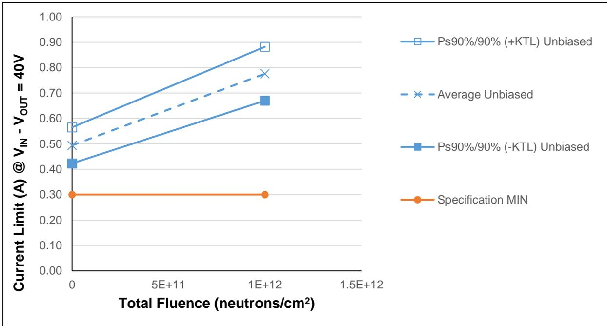
Figure 5.10: Plot of Current Limit @  $V_{IN} - V_{OUT} = 40V$  versus Total Fluence
