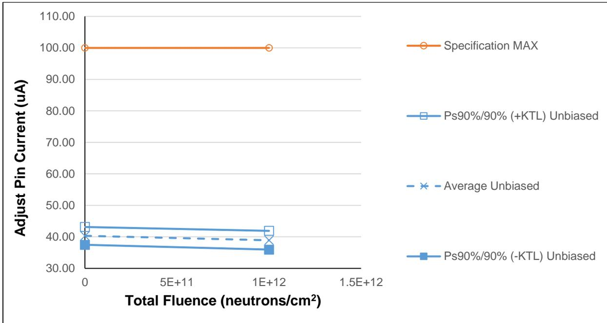
Figure 5.5: Plot of Adjust Pin Current versus Total Fluence
