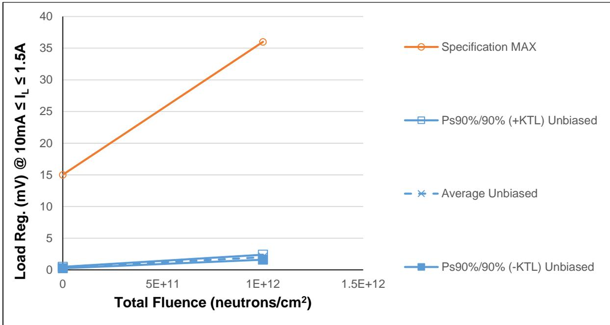
Figure 5.3: Plot of Load Regulation @  $10\text{mA} \leq I_L \leq 1.5\text{A}$ ,  $V_{OUT} \leq 5\text{V}$  versus Total Fluence
