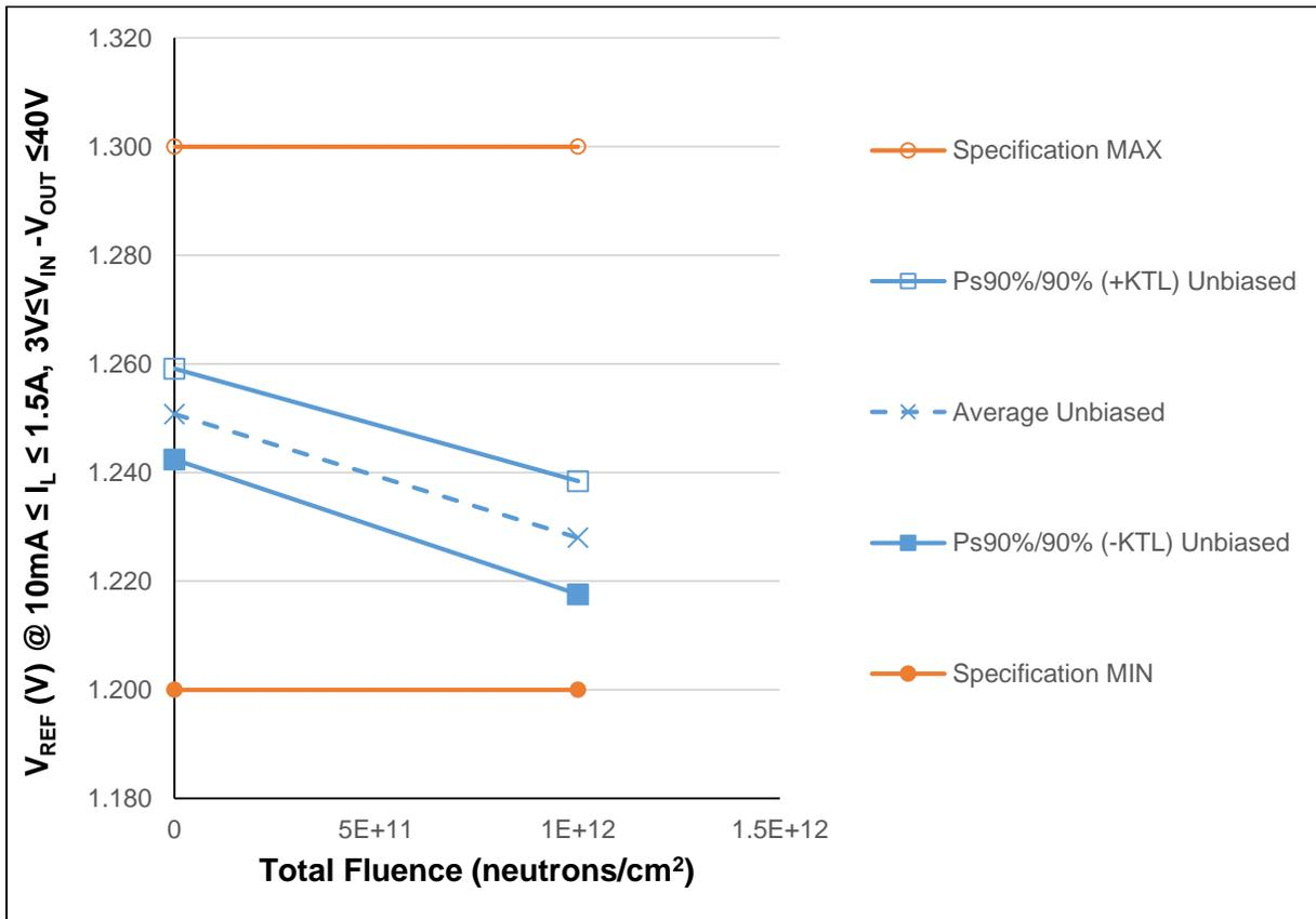
Figure 5.1 Plot of Reference Voltage @  $10\text{mA} \leq I_L \leq 1.5\text{A}$ ,  $3\text{V} \leq V_{IN} - V_{OUT} \leq 40\text{V}$  versus Total Fluence
