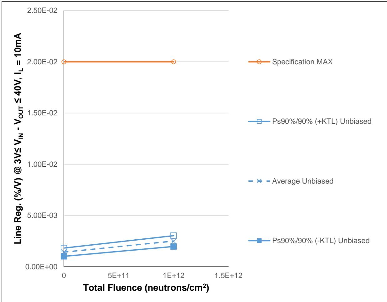
Figure 5.2: Plot of Line Regulation @  $3V \leq V_{IN} - V_{OUT} \leq 40V$ ,  $I_L = 10 \text{ mA}$  versus Total Fluence
