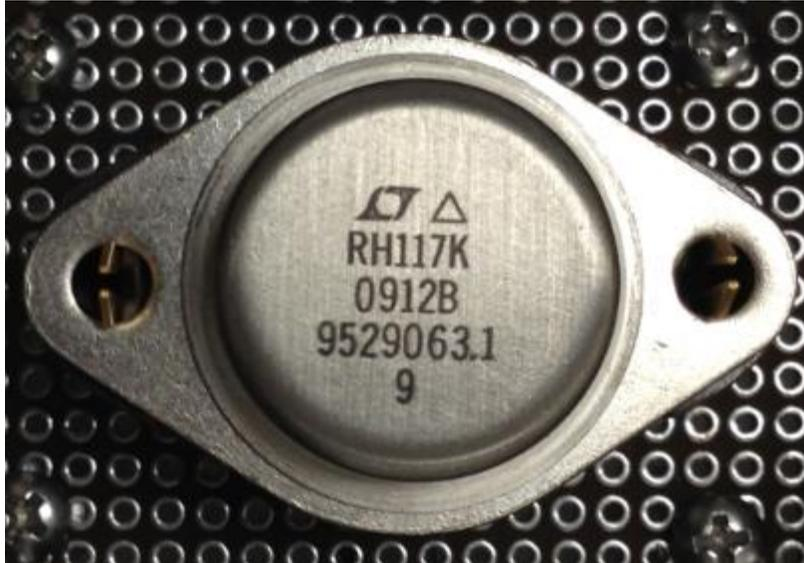
Figure A1: Top View showing date code, lot and wafer numbers
