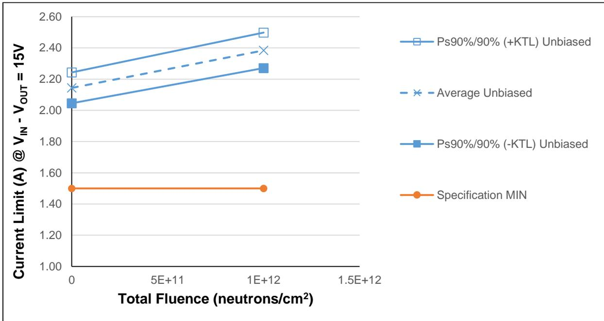
Figure 5.9: Plot of Minimum Load Current @  $V_{IN} - V_{OUT} = 15V$  versus Total Fluence
