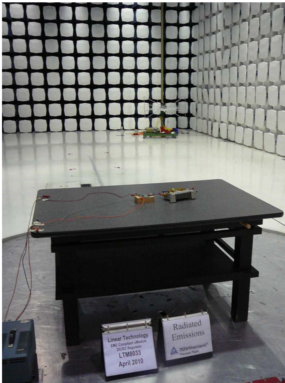
Figure 13 – Radiated Emissions 30 - 1000 MHz CFG3 Test Setup – Back
