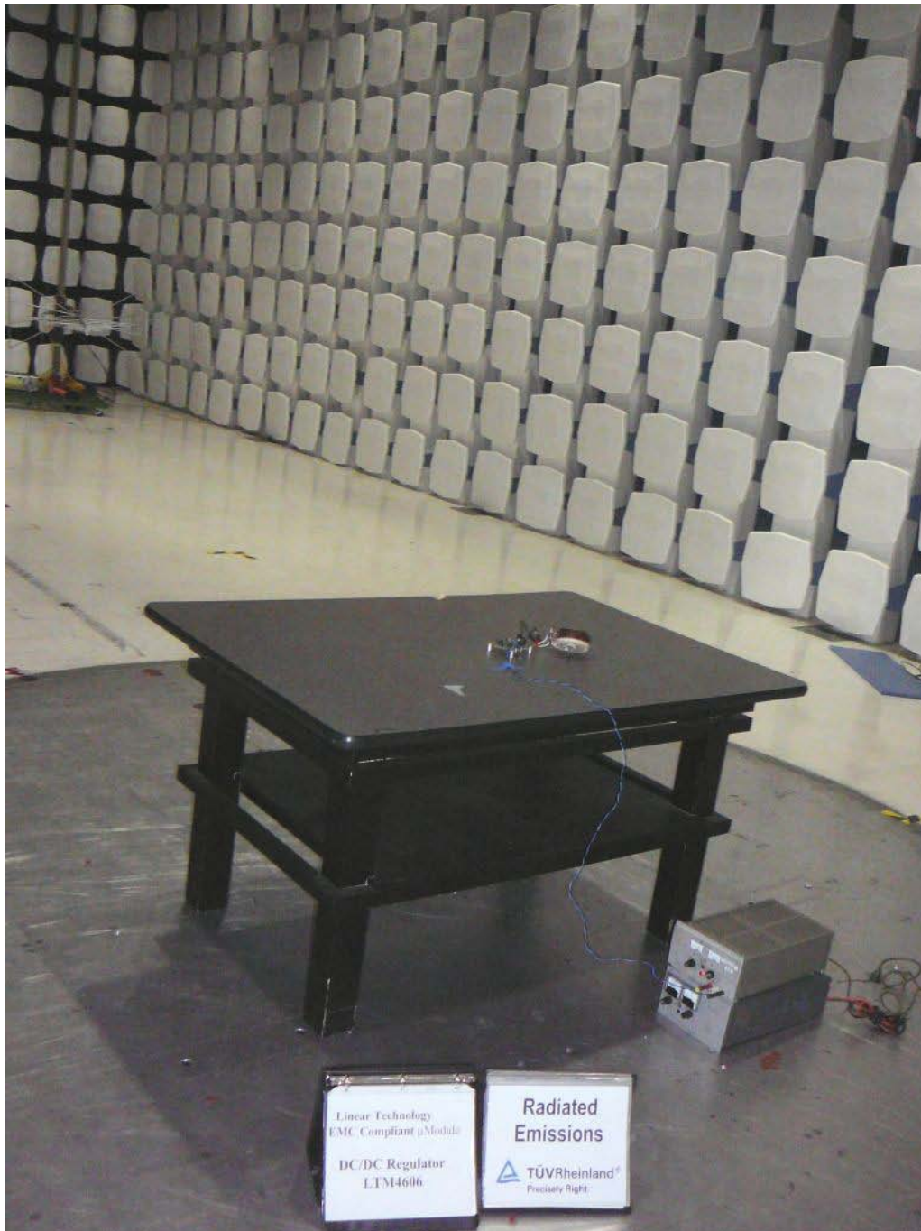
Figure 4 – Radiated Emissions 30 - 1000 MHz Test Setup – Back
