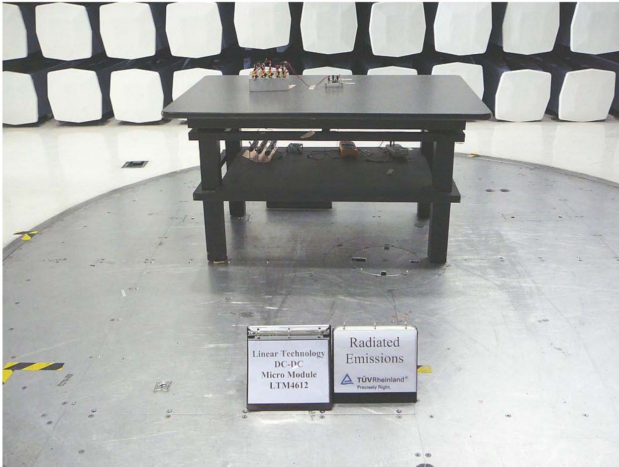
Figure 5 – Radiated Emissions 30 - 1000 MHz Test Setup – Load 2 – Front
