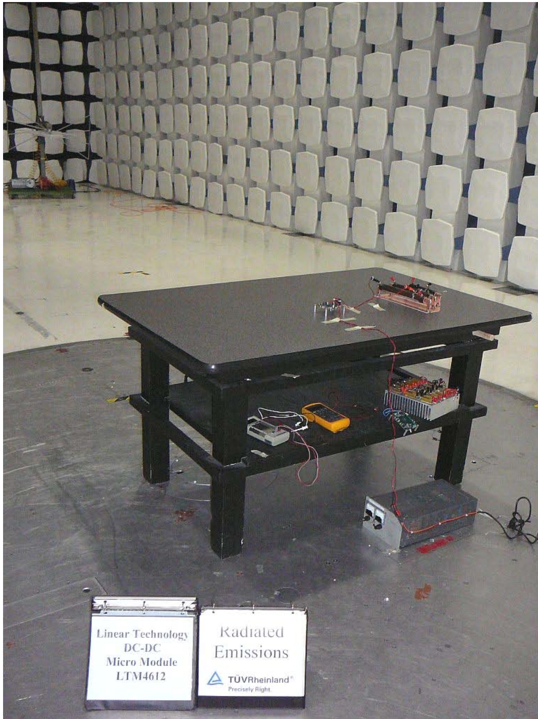
Figure 5 – Radiated Emissions 30 - 1000 MHz Test Setup – Load 1 – Back
