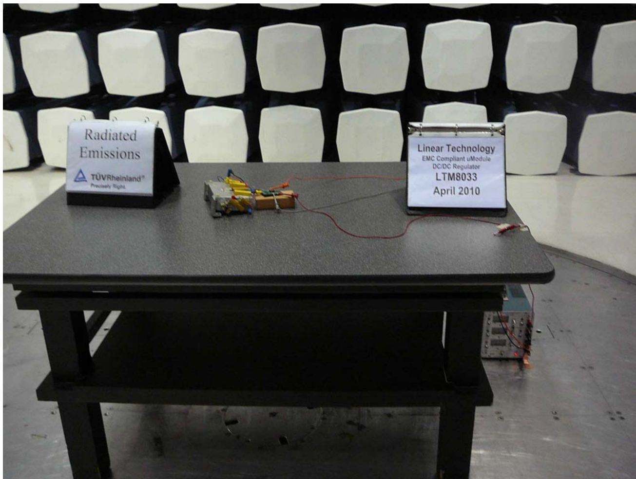
Figure 12 – Radiated Emissions CFG3 Test Setup – Front
