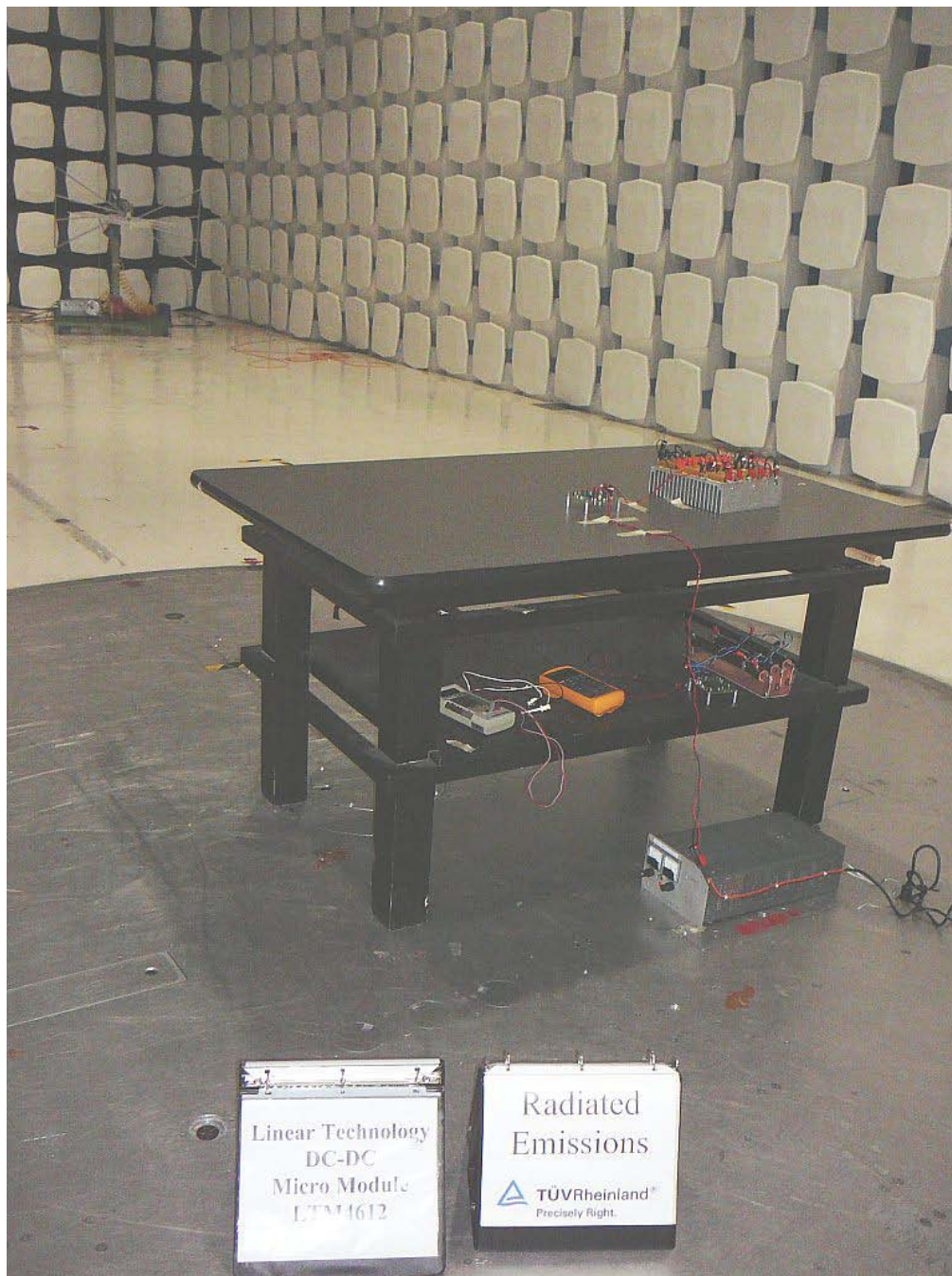
Figure 4 – Radiated Emissions 30 - 1000 MHz Test Setup – Load 2 – Back
