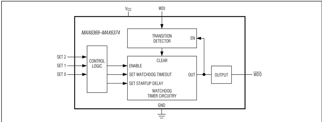
Figure 1. Functional Diagram
