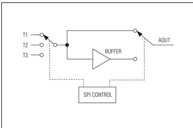
Figure 8. Analog/Temperature Measurement
