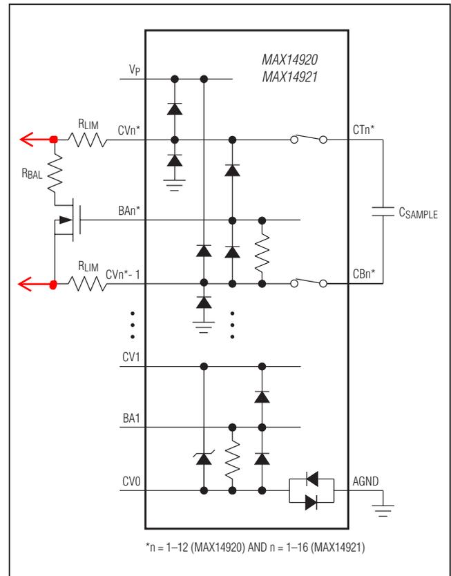
Figure 10. Input-Voltage Clamp
