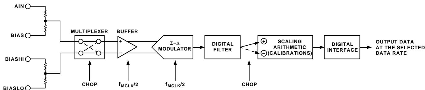
Figure 24. Channel Signal Chain Diagram with Chopping Enabled
