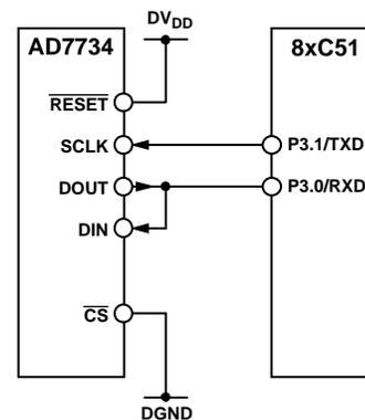
Figure 15. AD7734 to Host Device Interface, 2-Wire Configuration
