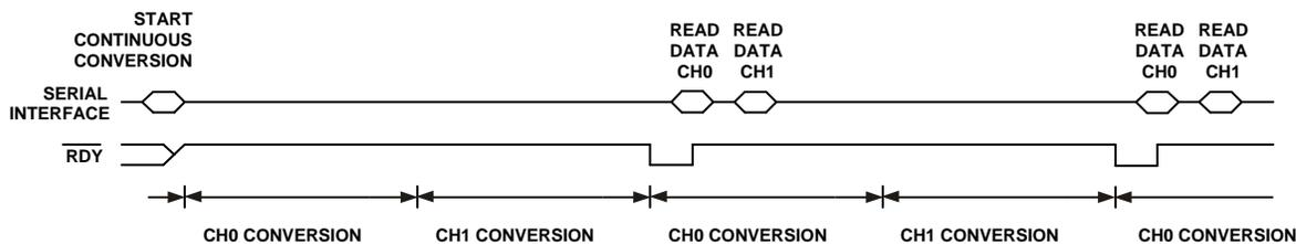
Figure 20. Continuous Conversion, CH0 and CH1, RDYFN = 1
