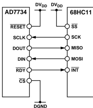
Figure 13. AD7734 to Host Device Interface, SPI
