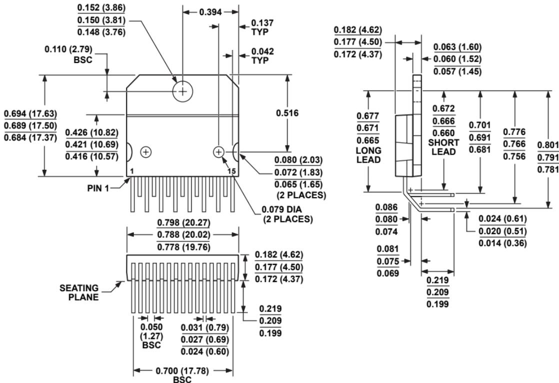
**CONTROLLING DIMENSIONS ARE IN INCHES; MILLIMETER DIMENSIONS
